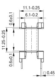
Hole arrangement View in mounting direction
