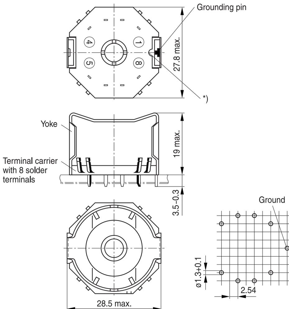
\*) This recess must be on the side of the grounding pin to ensure that the yoke locks into position.
