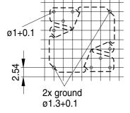
Hole arrangement View in mounting direction
